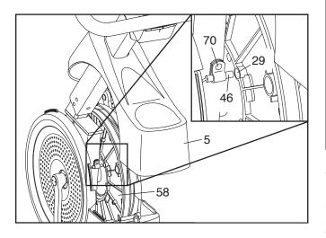
Locate the Reed Switch (46). Turn the Pulley (58) until a Magnet (29) is aligned with the Reed Switch. Next, loosen, but do not remove, the indicated M4 x 13mm Flange Screw (70). Slide the Reed Switch slightly closer to or away from the Magnet, and then retighten the Screw. Plug in the power adapter and turn the Pulley for a moment. Repeat these actions until the console displays correct feedback. When the reed switch is correctly adjusted, reattach the shield cover.
